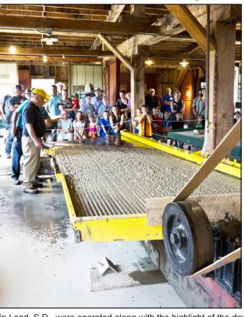
Left: The Western Museum of Mining & Industry (WMMI) ated a variety of equipment and provided blacksmith demonstrations and classes on Aug. 25. The Wilfley Shake Table shown above is the final stage in ore separation, using a violent shaking motion and water to further separate minerals other materials in the ore. The 1920 Osgood Steam Shovel, used to mine hematite in Wyoming, and the H.K. Porter trammer, which operated at the Homestake Mine
