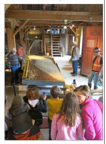
Above: Visitors to the 51st Annual Pikes Peak Gem and Mineral Show watch a demonstration of the museum's Stamp Mill. The stamp mill originally processed silver ore in the Montezuma area by first pulverizing the ore through stages and then separating out the minerals using mercury and the pictured shake table. For the demonstration, staff from the Broken Handle Mining Co. processed gold ore from the Hidee Mine near Central City. *Photo by David Futey*.
