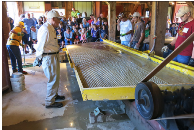
Above: Inside the WMMI’s Yellow Jacket Stamp Mill, a Wilfrey Shake Table is the last step in the ore separation process. The table violently shakes to settle denser minerals, and water is used to remove lighter sediment.
